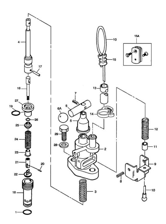
FIGURE 5 - LANYARD OPERATED PILOT VALVE
