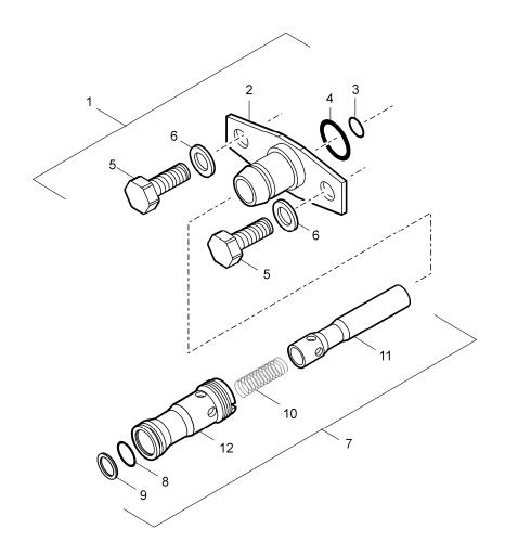
FIGURE 9 - AIR/FUEL PILOT VALVE CONNECTOR ASSEMBLY - OPTION "X"
