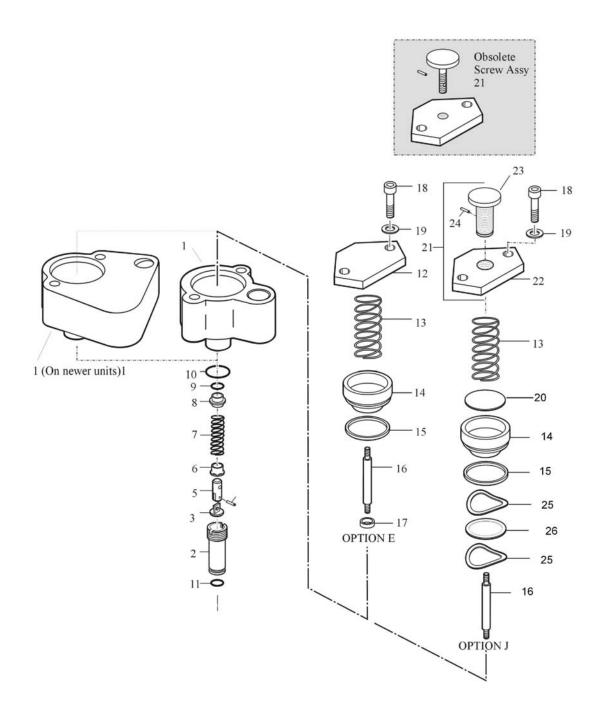
FIGURE 6 - AIR OPERATED PILOT VALVES
