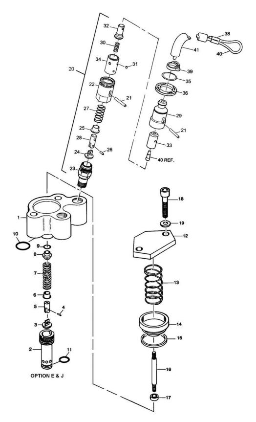
FIGURE 7 - AIR/LANYARD OPERATED PILOT VALVE, OPTION F
